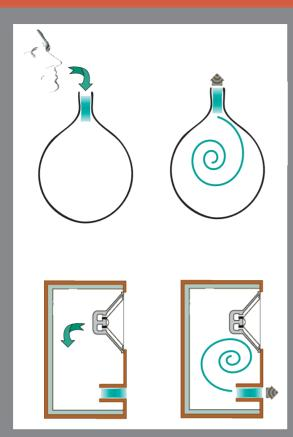
A simple Helmholtz resonator is a bottle with a narrow neck. Blow across it and you push the mass of the air in the neck of the bottle in, whilst the springiness of the air in the bottle pops it out again setting up an oscillation. Substitute your breath for a drive unit and the bottle neck for a port and you have a bass reflex speaker.
